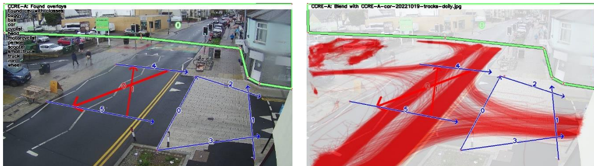
Figure 20: Constraints to vehicle path, Glamorgan Street (Cardiff)
