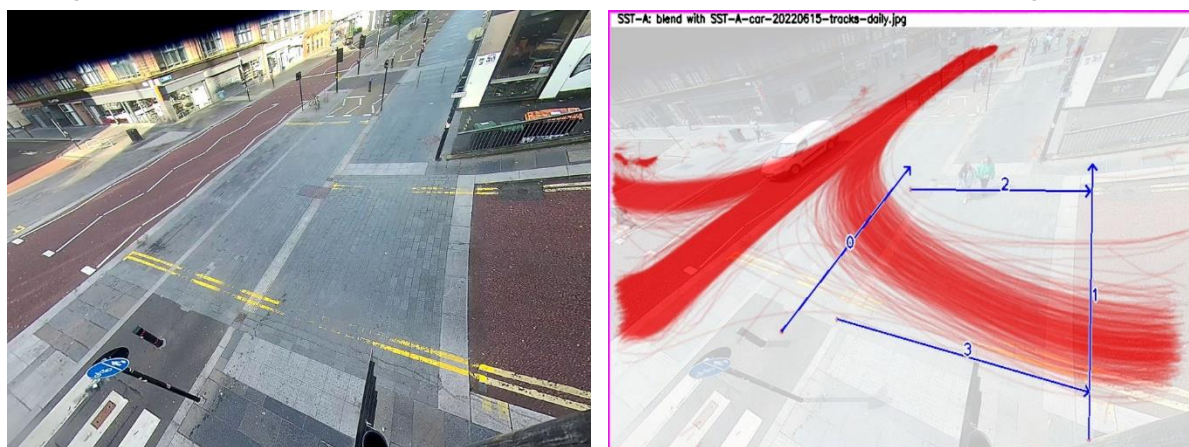
Figure 19: Problems with lack of constraint on vehicle path, Scott Street (Glasgow)
